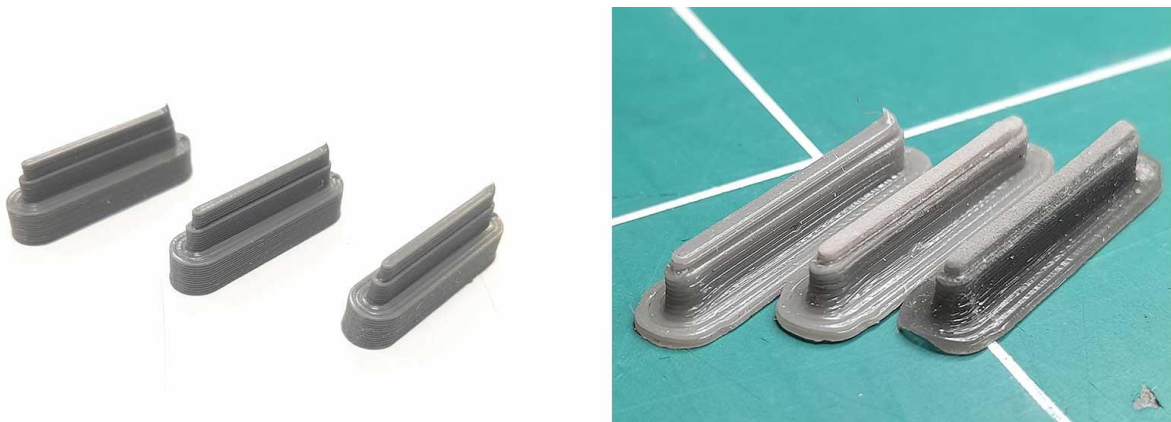
Silicone printed masking tools before and after zero, one and two plasma spray cycles.
